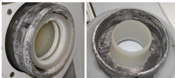
Figure 5: Corroded rotary seals on AES Baseline EP tool.
