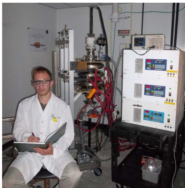
Figure 5: Initial vertical electropolishing trials with Oak Ridge National Laboratory three-cell cavity.
