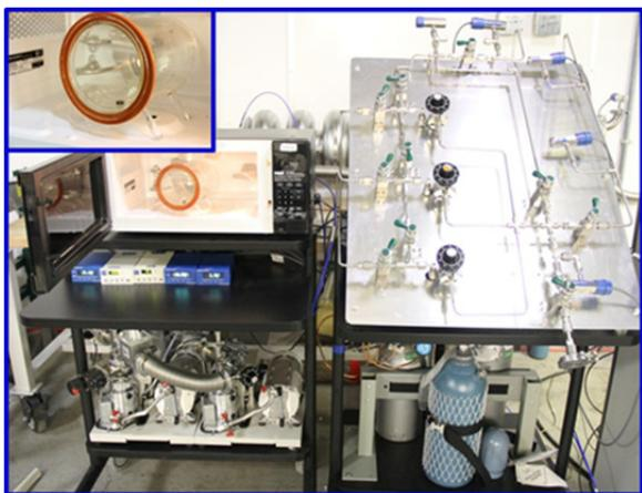
Figure 1: Microwave plasma processing set-up with gas feed system (sample inside the barrel is shown in inset).
