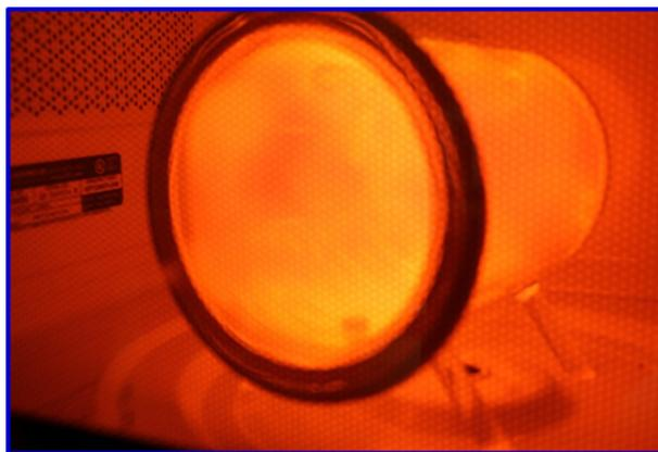
Figure 2: Ne plasma ignited in the microwave plasma reactor.
