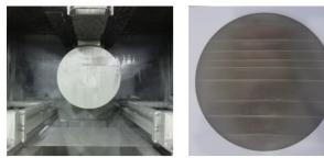
Figure 5: (Left) Slicing large grain Nb ingot by a multiwire saw and (right) one sliced large grain disk.
