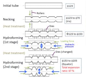
Figure 11: The fabrication process of hydro-formed seamless cavity from a seamless Nb tube.
