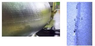
Figure 17: The outer surface (left) and inner surface (right) after barrel polishing of the W-1 cavity.
