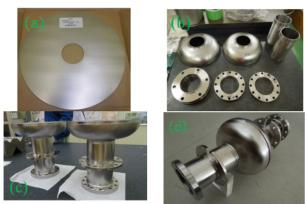
Figure 2: (a) Fine grain Nb disk, (b) cavity components before welding, (c) end groups and (d) completed cavity.
