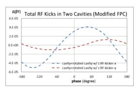
Figure 8: Cavity and rotated cavity arrangement (up) and the two cavities RF kicks (down).
