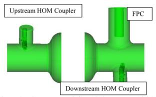
Figure 2: The upstream (left) and downstream (right) HOM/FPC couplers.
