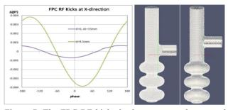
Figure 7: The FPC RF kicks in the current and proposed designs. d is the distance between the antenna tip and the beampipe wall.
