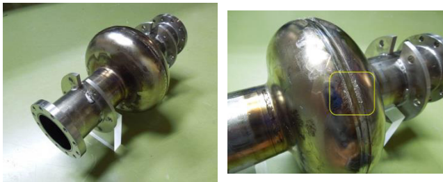
Figure 5: 1-cell cavity made by low RRR large grain Nb (left). On the equator part, several spatter marks are remained (right).
