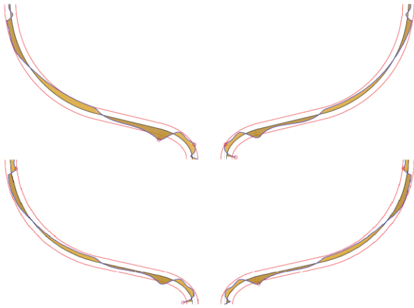
Figure 7: Representation of the measured cavity profiles. The red lines show the tolerance.
