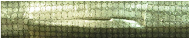
Figure 8: The pressure of the tube hydroforming process was incrementally increased until the tube cracked. This image shows the crack.
