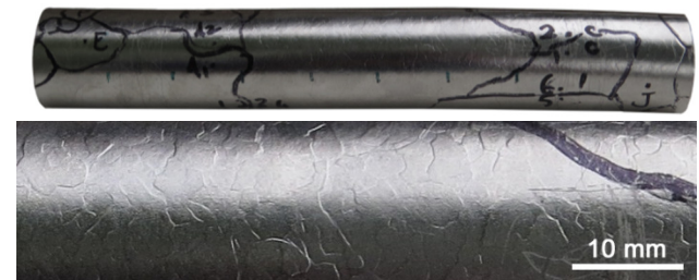
Figure 1: The large grain Nb tube. In addition to deeply grooved grain boundaries marked with black ink, the lower enlargement shows evidence for smaller grains with a few mm dimension at some point prior to growing the large grains.
