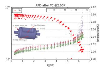
Figure 4: Local heating in the RFD as field is increased.
