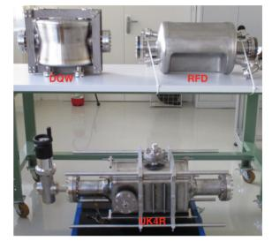
Figure 1: Picture of the crab cavities at CERN.
