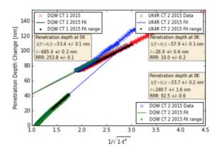
Figure 7: The change in penetration depth as a function of temperature  $(t = T/T_c)$ , with  $\lambda(T = 0, l)$  penetration depth, mean free path and RRR extracted for the DQW (baked [CT1] and unbaked [CT2]) and for the baked UK4R.
