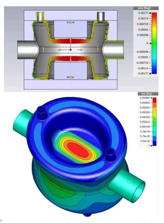
Figure 5: Cavity wall deformation due to radiation pressure at nominal deflecting voltage of 3.34 MV (CST simulation).
