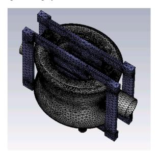
Figure 4: Mesh generated for structural simulation in CST MPhysics solver.
