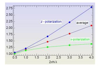
Figure 4: RF loss enhancement for sinusoidal surface variations with two H field polarizations.
