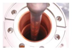
Figure 5: Example of copper oxidation.
