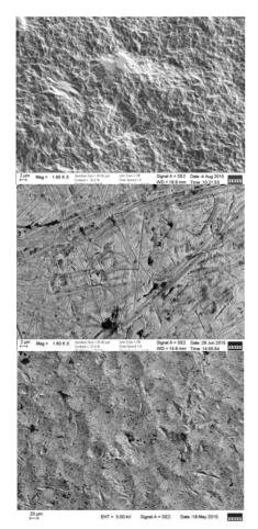
Figure 3: SEM photos of  $150 \mu m$  thick copper plating: (top) bellow with no post processing, (middle) Mo wool polished bellow and (bottom) bead blasted coupon.
