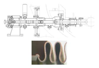
Figure 1: (top) TTF-3 coupler, (bottom) sectioned inner bellows after plating to 150 µm thickness.
