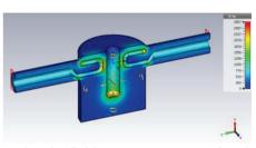
Figure 9: Electric field map at 400MHz for the RFD FPC test box. (Absolute magnitude, linear scale).
