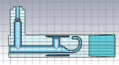
Figure 12: The DQW HOM coupler terminated into a 70 mm long conical SiC absorber with radii 31mm and 28 mm.
