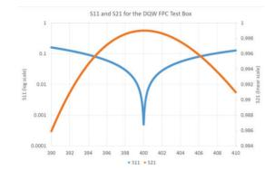
Figure 6: The reflection coefficient for the DQW FPC test box over a 20MHz span centered on the operating frequency.
