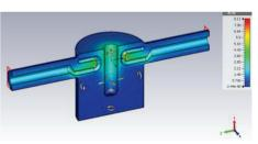
Figure 10: Magnetic field map at 400MHz for the RFD FPC test box. (Absolute magnitude, linear scale).
