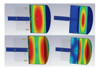
Figure 19: Manipulation of the  $TE_{111}$  mode from 500MHz (left) to 812MHz (right) through use of the variable plate (Electric field top, magnetic field bottom).
