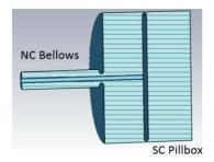
Figure 18: A basic model of a variable pillbox cavity. The section on the left contains the normal-conducting bellows, and no field. The section to the right is the superconducting region of high field where the couplers will be positioned.
