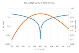
Figure 11:  $S_{11}$  and  $S_{21}$  for the RFD FPC test box over a 20MHz span centered on the operating frequency.
