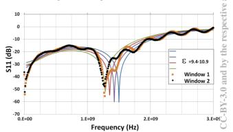
Figure 3: Measured (black and orange dots) and calculated reflection coefficients for two RF windows with the  $\overline{\sim}$ 'hourglass-shaped' central conductor
