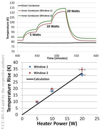
Figure 5: Top – temperature rise due to conduction in alumina and copper, bottom – analytically calculated versus measured termperature increase.
