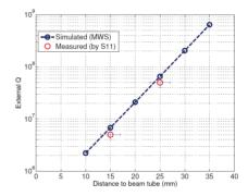
Figure 5: Measured v.s. simulated  $Q_{ext}$  of the quarter-wave coaxial coupler.
