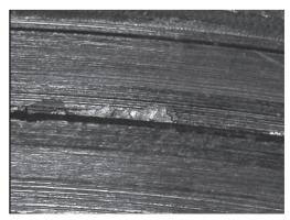
Figure 6: Microscopic picture of the knife edge of the hardened Nb1Zr flanges.
