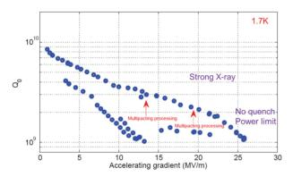
Figure 7: The  $Q_0$  vs  $E_{acc}$  of the coupler cavity.
