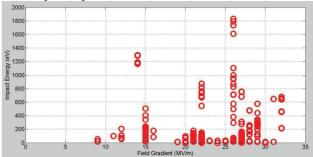
Figure 8: The impact energy vs  $E_{acc}$  of the coupler cavity.
