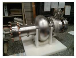
Figure 4: The quarter-wave coaxial couple with a single cell cavity.
