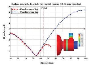
Figure 3: The magnetic field distribution on the surface of coaxial coupler with insert (with  $E_{acc} = 31.5 \text{ MeV/m}$ ).
