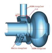
Figure 1: Schematic of Euclid proposed quarter-wave coaxial coupler.
