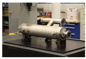
Figure 2: LCLS-II cavity/ helium vessel inspection.
