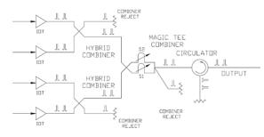
Figure 1: IOT combination scheme used in each of the Diamond 300 kW amplifiers.
