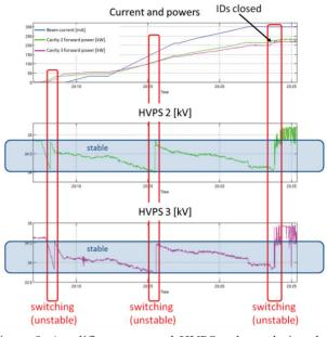
Figure 9: Amplifier power and HVPS voltage during the fill of the storage ring.
