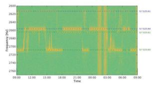
Figure 6: Intensity jumps in horizontal spectrum corresponding to changes in the number of active modules.
