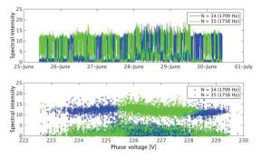
Figure 5: Relative intensity of two rotation lines (upper) and the dependence of line intensity on phase voltage (lower).
