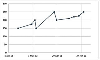
Figure 5: Peak beam current over time after cavity module replacement in January 2013.
