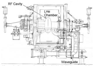
Figure 3: Cutaway view of the CESR-B SRF cryomodule.
