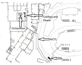
Figure 2: The 52 m MCTL layout for the existing system.
