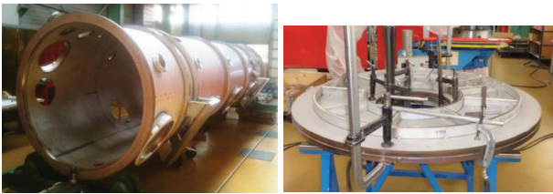
Figure 6: Picture of the vacuum vessel tube (left) and lid (right) under manufacturing.
