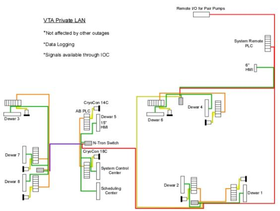
Figure 4: VTA controls, physical layout.
