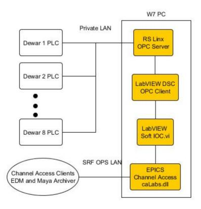
Figure 5: VTA controls, software layers.
