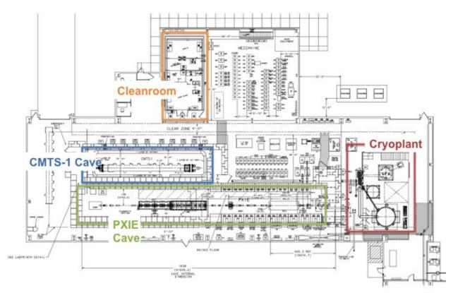
Figure 5: Layout of CMTF. The Cryomodule Test stand is outlined in blue, Cryoplant area in red, PXIE enclosure in green, and Cleanroom in orange.
