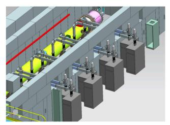
Figure 3: RF layout for testing LCLS-II 1.3 GHz cryomodules.
