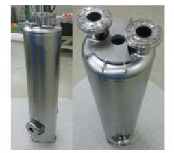
Figure 3: Quarter wave resonator after final electron beam welding.
