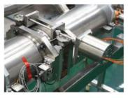
Figure 4: Tuner and piezo.
