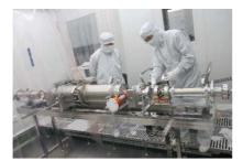
Figure 3: Cavity beamline assembly in clean room.
