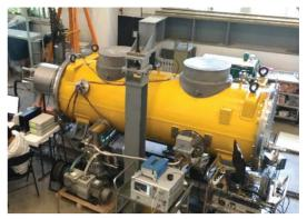
Figure 5: Assembled cryomodule.
