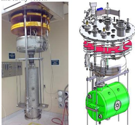
Figure 8: FRIB production insert design.
