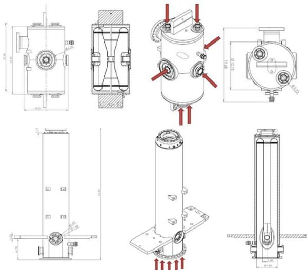
Figure 5: Cleaning access for HWR and QWR.
