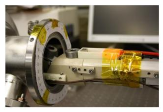
Figure 3: XRF probe entering the inner space of a 9-cell cavity.
