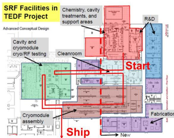
Figure 1: Work Flow for CM Production.
