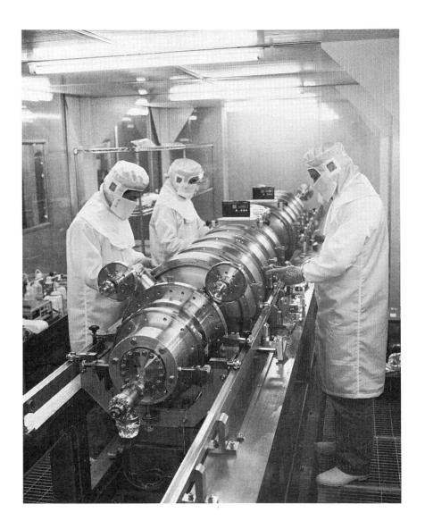
Fig.6 Cavity assembling in the clean room.
