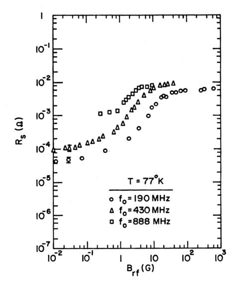
Figure 6 - Superconducting surface resistance of bulk YBCO measured at several frequencies and temperatures. A peak rf field of more than 600 gauss was obtained at 77 K.
