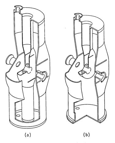
Figure 3. Conceptual design of (a) a coaxial half-wave resonator and (b) a coaxial quarter-wave resonator of frequency 352 MHz and particle velocity 0.12 c fabricated with high-conductivity sheet niobium.
