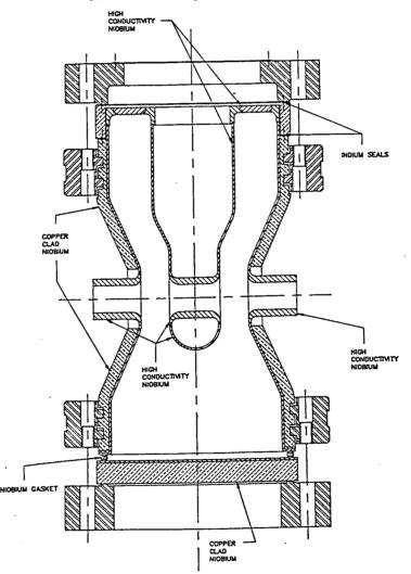
Figure 2. Coaxial quarter-wave resonator of frequency 425 MHz and particle velocity 0.155 c fabricated with a copper-clad niobium outer conductor.
