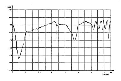
Fig.3 Transfer function of HOM coupler.
