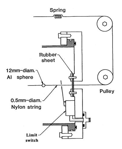
Fig.3 Cross-sectional view of the end beam-tube flange.
