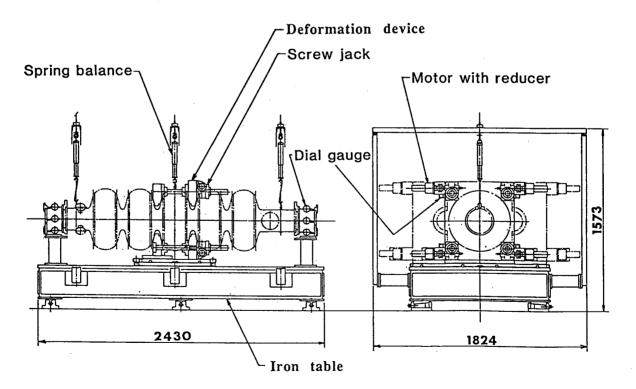
Fig.2 Pre-tuning instrument.
