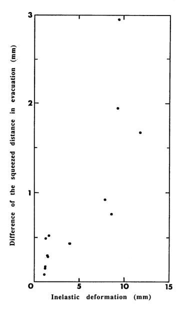
Fig.11 Difference of the squeezed distance in evacuation between before and after pre-tuning as a function of the total inelastic deformation length of each cavity.
