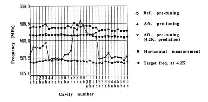
Fig.7 Resonant frequencies of the cavities before and after pretuning as well as that at horizontal measurements.
