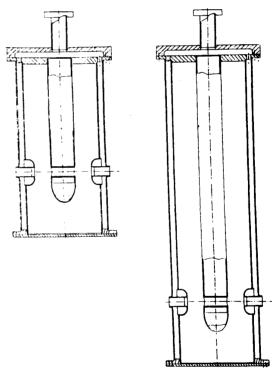
Fig. 4 Bulk niobium cavities: a) 160 MHz,  $\beta_o = 0.11$ ; b) 80 MHz,  $\beta_o = 0.055$ .
