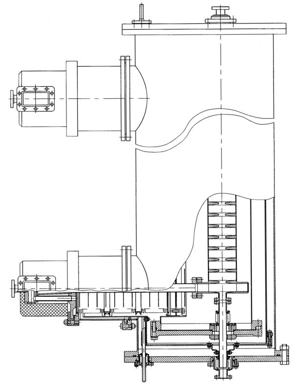
Fig.3: Design of the cryostat with the accelerating structure
