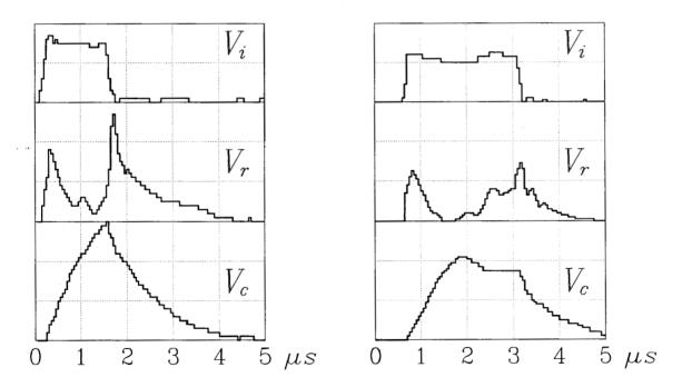
Fig.7: Pulse patterns of the incident wave field, the reflected wave field and the cavity field.
