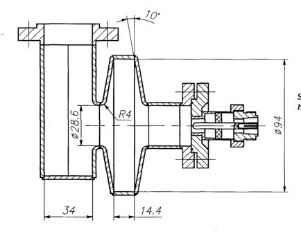
Fig.5: Single cell cavity for high power pulse tests.
