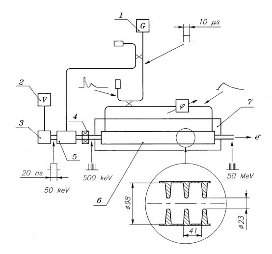
Fig.1: Skeleton diagram of linear accelerator
