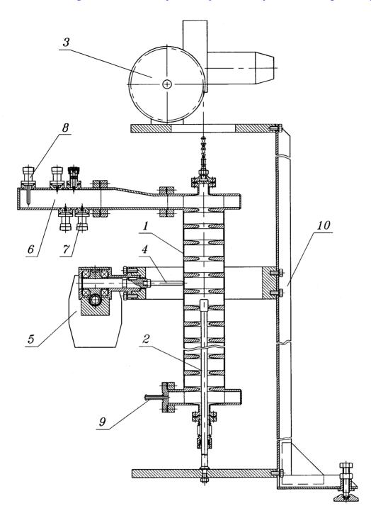
Fig.4: Design of the set-up for tuning the accelerating structure
