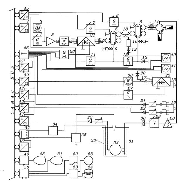
Fig.6: Block diagram of the setup for single cell cavity tests
