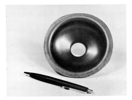
Fig.4 Half-cell of the RF-structure after deep-drawing.
