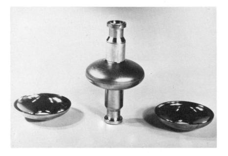
Fig.5  $E_{0,1}$ -cavity and two half-cells after locks fabrication.
