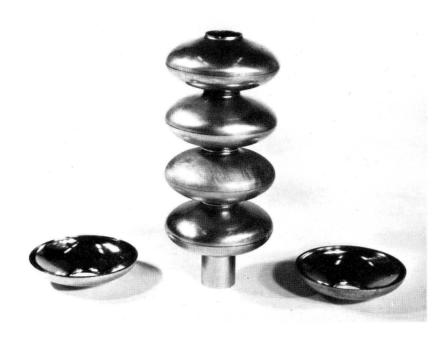
Fig.6 Superconducting RF-structure made of Nb sheet prior to welding.
