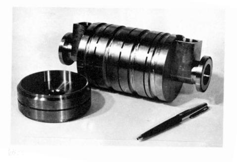
Fig.2 Capture section made from casted Nb.
