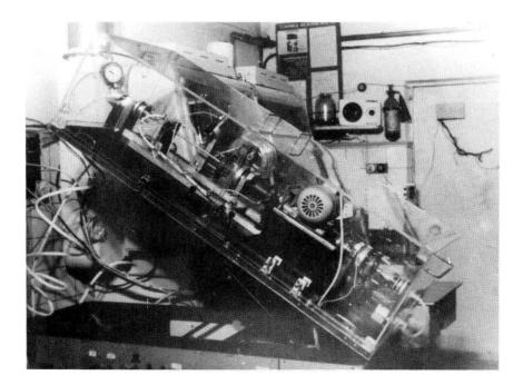
Fig.7 Instalation for electro-chemical polishing of RF-structures and  $E_{01}$ -cavities from niobium.
