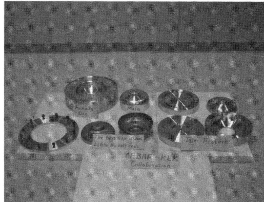
Fig.3 Dies for deep drawing and a set of trimming jigs.
