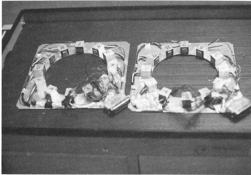
Fig.5 Array of PIN diodes for the radiation measurement. They were set on the beam duct adjoining the end module.
