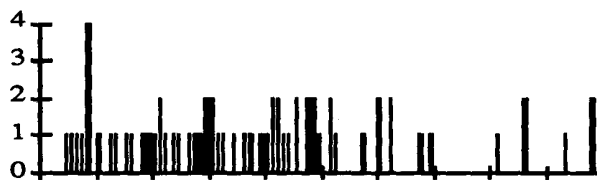
Fig. 2: Number of defects detected by "temperature-mapping" vs. consecutive test number. A defect is defined as inducing a temperature signal \Delta T \geq 100 mK.
