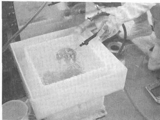
Fig. 3 Megasonic rinsing in the clean room.
