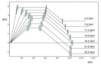
Figure 5: Schematic view of the spreader.
