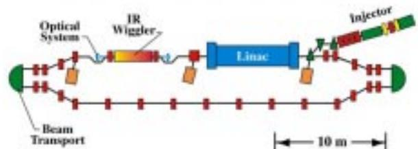
Figure 6. Schematic layout of the JLab IR FEL.
