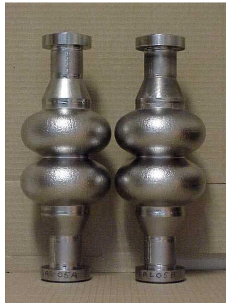
Figure 1: hydroformed 3 GHz bicells Nb cavities
