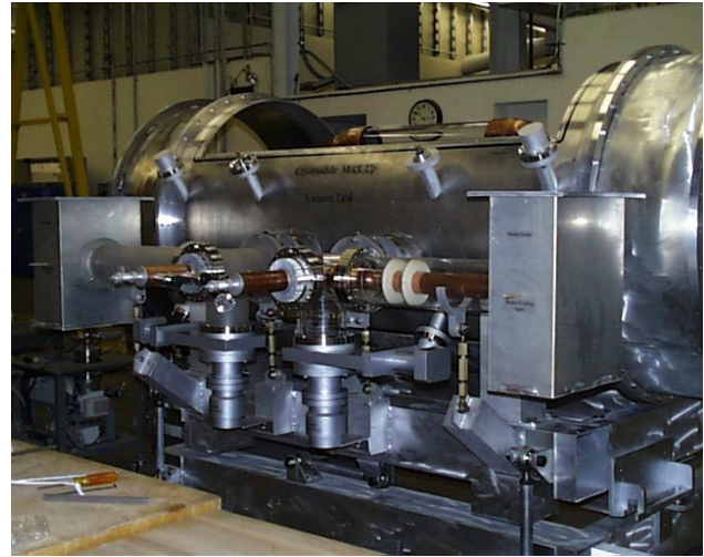
Figure 6: The mocked-up cryo-module is a full size model of the APT cryo-module for the \beta=0.64 cavities.
