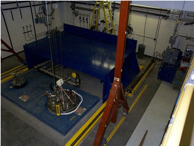
Figure 2: The movable radiation shield in the test area.
