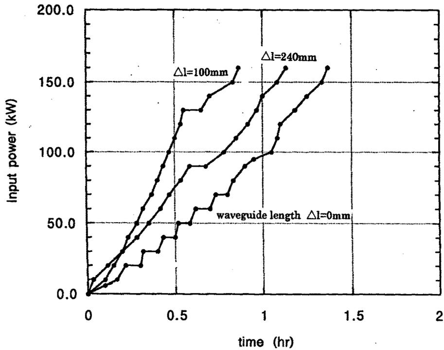
Fig. 6 total reflection test of ultra pure water rinsed Coupler
