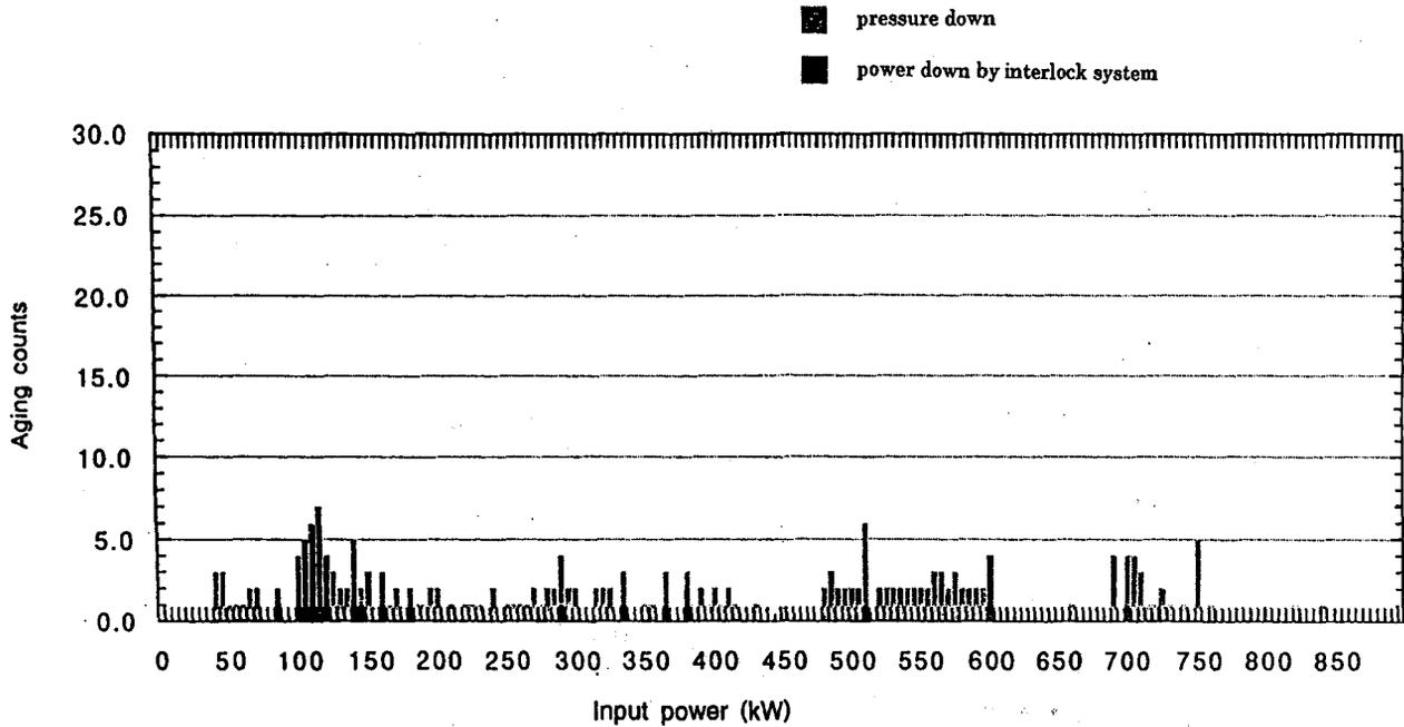
Fig.4 ozonized ultra pure water rinsed Coupler aging counts
