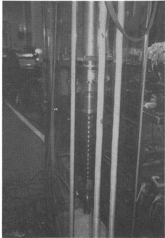
Fig. 1 Coaxial input coupler for KEKB SC cavities
