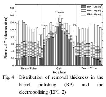
thickness at the equator (>100 $\mu$ m) is much larger than that at the iris and the beam tube (~20 $\mu$ m). On the other hand, the iris and the beam tube were polished much more than the equator by the EP1 and the EP2. Then, the total removals of ~140  $\mu$ m and ~80  $\mu$ m were achieved at the equator and the iris, respectively. It is noted that the BP is very simple method to remove mechanically the surface including welded area, while it requires a long period of about 10 days.
