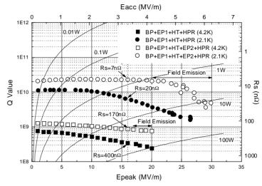
Fig. 5 Q values of the  $\beta$ =0.5 single cell cavity as a function of peak surface electric field (E<sub>peak</sub>)
