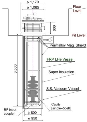
Fig. 2 Schematic view of the cryostat
