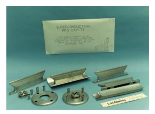
Figure 4. View of the Niobium RFQ electrodes of the Los Alamos four vanes model before the welding.( Courtesy of Dr. James Stovall )
