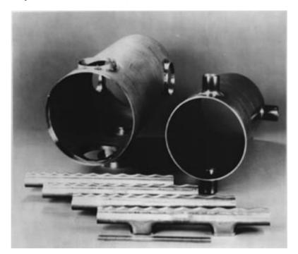
Figure 5. View of the electrodes and the external jackets before the final welding. ( Courtesy of Dr. Kennet Shepard )
