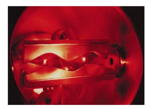
Figure 3. Bottom view of the SUNY SRFQ resonator
