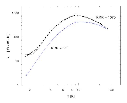
Fig. 8: Heat conductivity versus temeperature for niobium.
