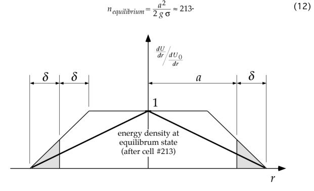
Fig. 4: Energy loss after cell number 213 (quasi equilibrium state).
