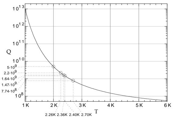
Fig. 10: Quality factor versus temeperature. The unloaded Q is assumed to be  $5*10^9$  (RRR=300).
