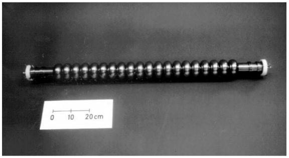
Figure 3: Photograph of a 20-cell cavity operating at 3 GHz. The cavity consists of 18 identical center cells and two endcells which compensate the influence of the attached beam tubes.
