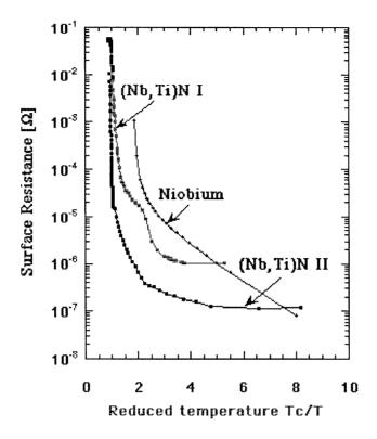
fiFig 1; Comparison between the surface resistance of 3 GHz (Nb-Ti)N cavities and Theoretical BCS Surface resistance versus  $T_C/T$  of the Nitride. The Critical Temperature  $T_C$  of the Nitride was 17.1 K.
