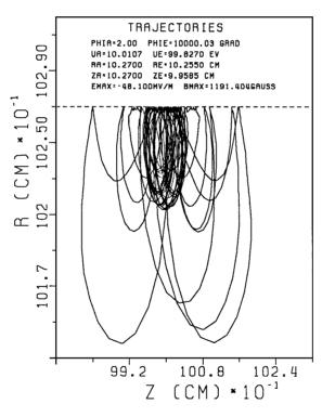
Fig 3; Two point Multipacting at the equator of a 1.3 GHz spherical cavity; the Accelerating field is 25 MV/m
