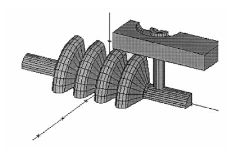
Fig 5; Design of the prototype cavity equipped with the main coupler
