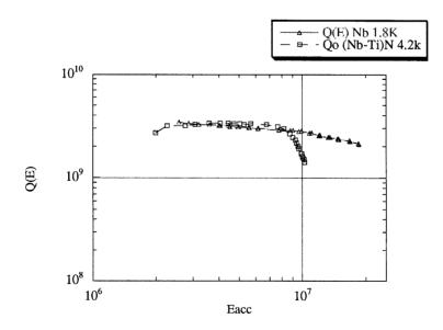
Fig 2, Comparison between Quality factor versus field of two 3 GHz cavities built in (Nb-Ti)N and niobium
