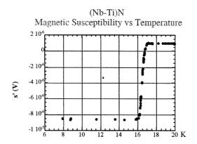
Fig.4 AC Magnetic susceptibility of Niobium Titanium Nitride showing only a clean 17.1 Tc phase on the sample surface
