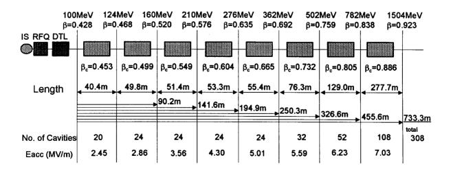
Fig.1 Preliminary conceptual design of the superconducting linac.
