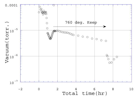
Fig. 2. Annealing condition of cavity.
