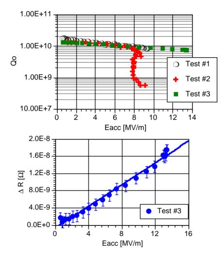
Figure 1: Performance of cavity K–15; the slope in  $Q_0$  vs  $E_{acc}$  in test #3 is caused by an additional resistance  $\sim E_{acc}$ .
