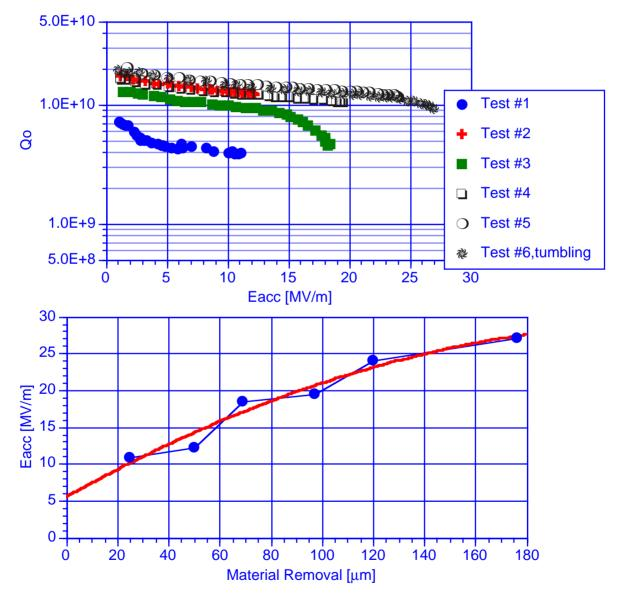
Figure 3: Dependence of achievable gradient on amount of material removal, measured on cavity K–17.
