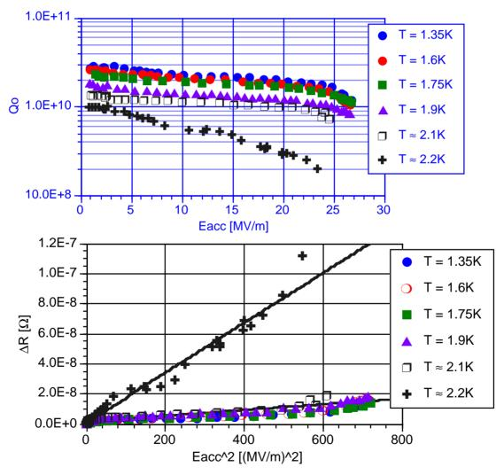
Figure 4: Results from tests on cavity JL–1. The slope in Q<sub>0</sub> vs  $E_{acc}$  is caused by an additional resistance  $\Delta R \sim E_{acc}^2$ . The change in slope around  $T_{\lambda}$ points to a heat transfer problem at the defect.
