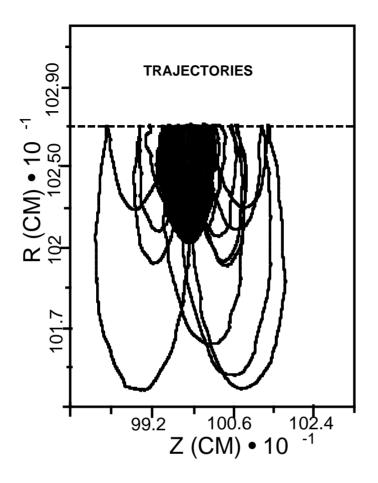
Figure 6:2–point multipacting at  $E_{acc} \approx 25 MV/m$ , corresponding to a peak magnetic field of  $H_{peak} \approx 1100$  Gauss at the equator of the cavity.
