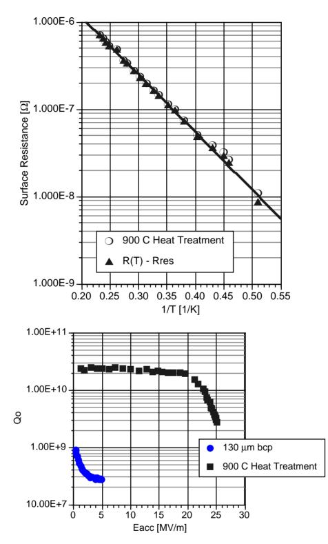
Figure 2: Performance of cavity K–16. Strong Q-disease was seen immediately after barrel polishing and chemical treatment. After hydrogen degassing at 900° C a residual resistance of  $R_{res}$ =2.2 n $\Omega$  was achieved and gradients up to  $E_{acc}$ =25MV/m were measured.
